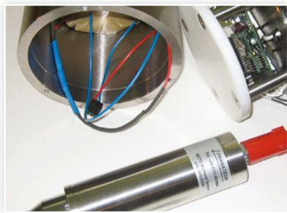
The FDL-Compact is a dedicated data logger for the operation of the METS. With integrated battery pack, it allows fully autonomous operation of one METS for up to 3 months.
